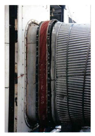
The PS-8306-01 is a replacement assembly for the Ruston TB series turbines using the TB-83006C molded exhaust joint.
