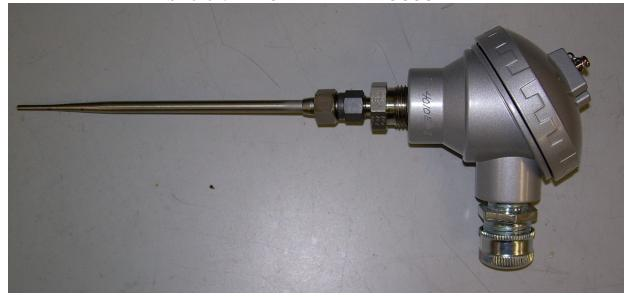
The PS-4010E/xx duplex thermocouple is a fit, form, and function replacement for the OEM original on TA and TB series turbines. This is a Type K thermocouple accurate to +/- 2 deg. F at Tmax. The duplex thermocouple is actually two thermocouples in one allowing dual monitoring functions, redundancy setup or the ability to changeover connections in the event one side fails.
