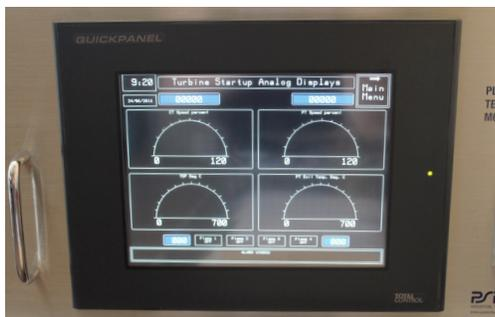
Turbine Startup Analog Displays Screen
