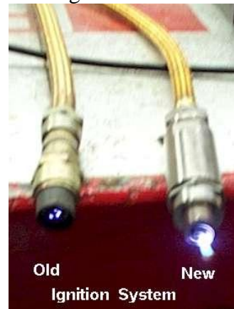
Booster coil (64/51001096) with a Lodge plug (TA-23119). Both old and new are powered by the same 24VDC power supply
